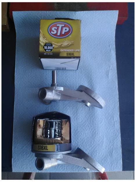
One solution to prevent this from happening is to cut the tip of the oil tube in a 45 degree angle, or if you experience this situation before, cut the oil tube ¼" with a tubing cutter. That space will prevent the overpressure valve from blocking the tube, and you will be on the safe side. I hope this Tech Tip help prevent another ruined engine.
