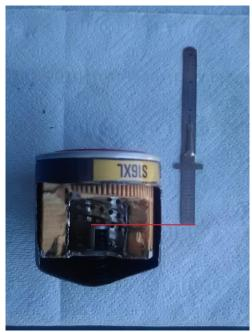
The red arrow shows the area where the overpressure relieve valve make contact with the oil tube blocking the oil going back to the engine. No oil pressure will be present or measure at the oil gage.
