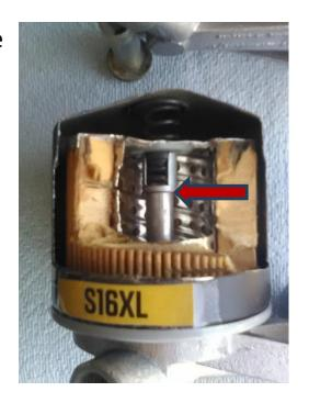
This is not the only filter with this situation. There are other brands with similar size but some have the overpressure valve located near the area of the threaded hole. Be careful when changing the oil filter in your MGB. If you don't get oil pressure in about 30 sec. when you start the engine after an oil change, Stop! and check the filter.
