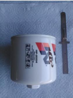
The filter shown below shows the over presure relief valve at the bottom of the filter not the canister, making it to short to clear the oil tube on the MGB oil adapter.
